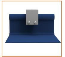
**Step 3:** Fasten clamp on side with 2 blind rivets.
