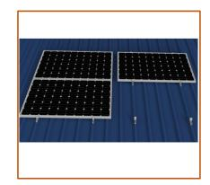
Step 4: Finish all solar modules installation one by one.
